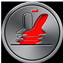
You must release and center (where applicable) the joystick/switches to resume normal operation. If you do not release within five seconds the powerchair will not be able to move, even if you release and operate it again. The screen will display a diagnostic screen at this time. You can reset this condition by switching the Bugzi off and on again.
