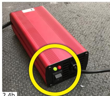
Always disconnect the mains supply before disconnecting the battery. Don't forget to replace Bugzi's power lead after charging!
