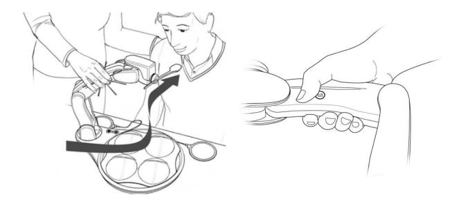
When the Teach Icon is covered, the Arm will be free for the Caregiver to move. The last two sections of the Arm will remain engaged and will keep the Spoon level when moving within the teach space. If resistance to movement is present, the thumb is probably not completely covering the Teach Icon.
