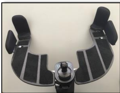
The pads are removable allowing for the placing of buttons or a Moozi Joystick if that is the way the child controls the WizzyBug
