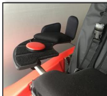
The pads are removable allowing for the placing of buttons or a Moozi Joystick if that is the way the child controls the WizzyBug
