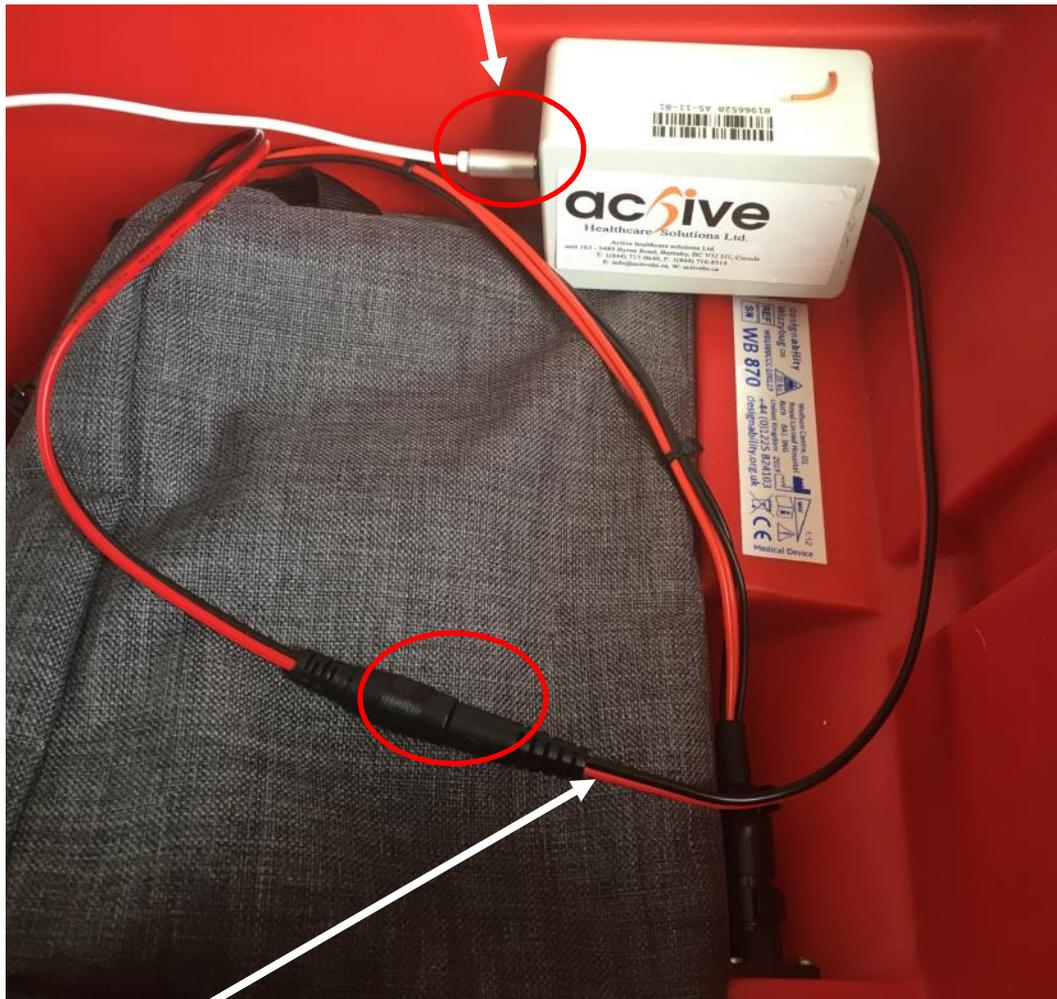
This cable plugs into female end of installed extra battery cable as shown.
