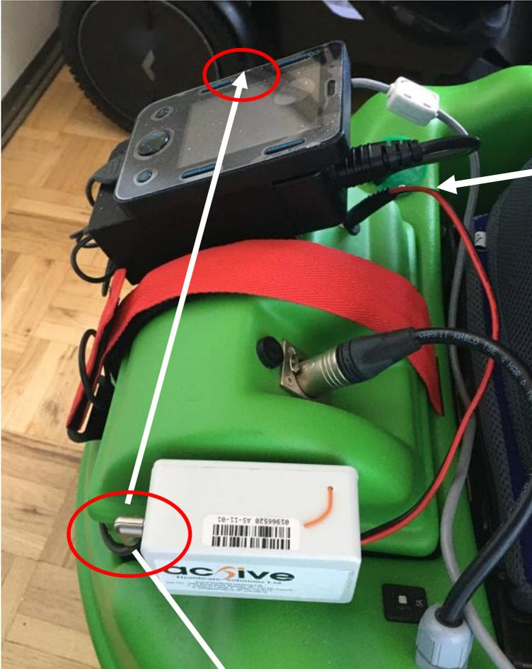
Red & Black Connector Cable from Kill Switch box goes to Bugzi Battery Box as shown.
